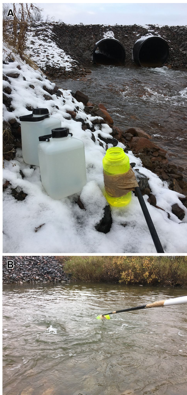
Fig. 2 Extendable pole with standard plastic sample container used to collect water samples according to the official protocols in the present study
